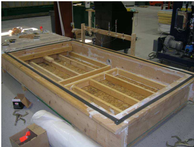
Figure 1. Pressure Chamber used for pressure testing. The blower is located in the upper right of the photo, with the linear displacement sensor rack and DAQ control computer in the upper center of the figure
