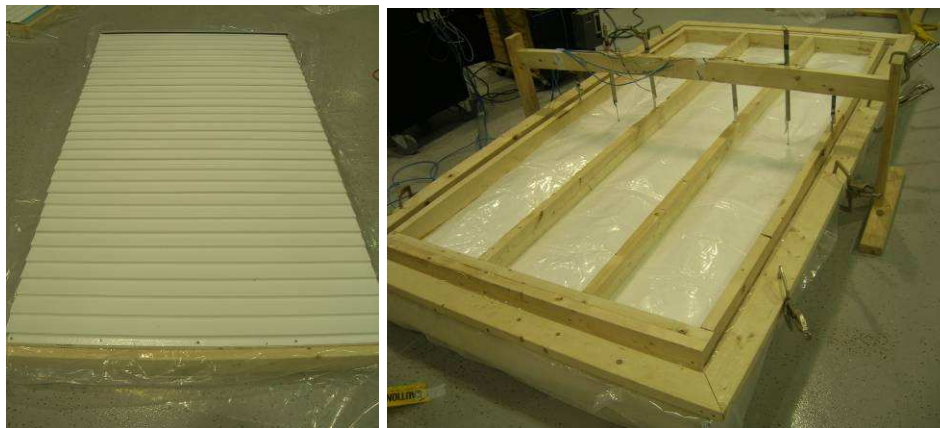
Figure 4. Negative pressure foam-vinyl test sample after assembly and loaded in chamber for testing
