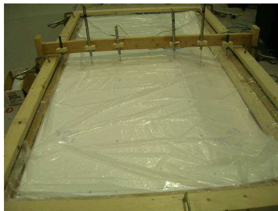
Figure 6. Failure in positive pressure test where foam pulled off fasteners on right end stud
