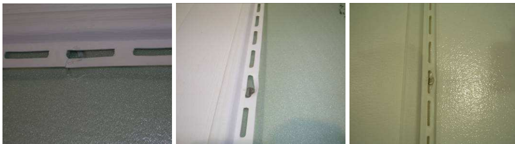
Figure 8. Negative system test failures (described from left): Siding tear from fastener, Siding disengagement from fastener, and siding partial disengagement from fastener
