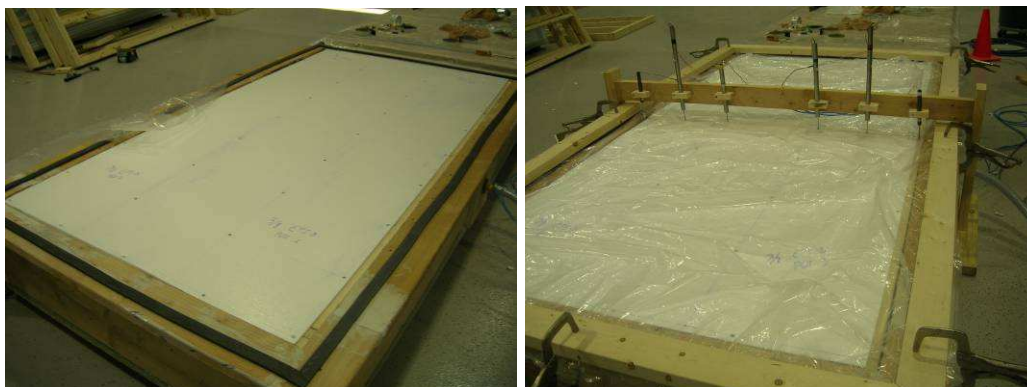
Figure 2. Foam sheathing prepared for positive pressure test
