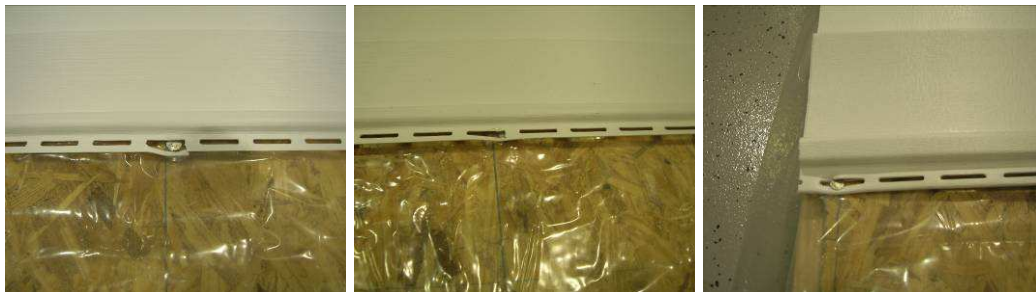
Figure 7. Baseline test failures (described from left): Nail hem tear, Siding disengagement from fastener, and partial disengagement from fastener
