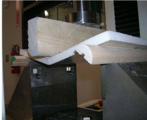
Figure 10. ISO sample undergoing flexural test
